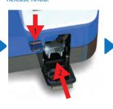
5) Pipette 60uL of Stained Sample Into the Cassette. Close Door. Test Begins.
